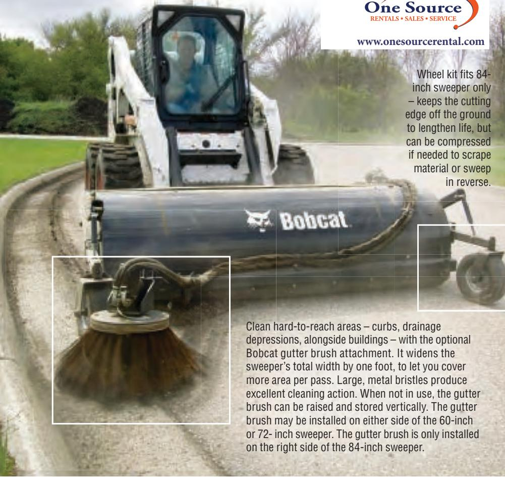
Wheel kit fits 84-inch sweeper only – keeps the cutting edge off the ground to lengthen life, but can be compressed if needed to scrape material or sweep in reverse.
